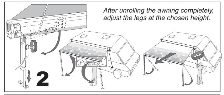
To avoid that the awning is lifted up by an unexpected gust of wind, it is necessary to secure the legs to the ground with the provided hooks. For greater safety, we strongly advise you also to use some storm cords in the upper part of each support leg or to anchor the awning with the Fiamma Tie-Down Kit strap.
