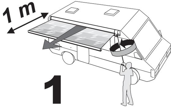
*In order to avoid unnecessary strain on the awning as well as on the vehicle side, we suggest to take out the legs at about 1m from the opening.*
