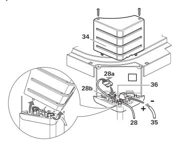
When power packs or power supply units are being used, note that the output voltage is between 11 V and 15 V and the alternating current ripple is < 1.2 Vpp. We recommend the automatic chargers from Truma for the different applications. Please ask your dealer. Other chargers may be used only with a 12 V battery as a buffer.
