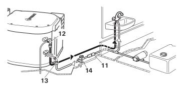
When using the Truma Ultrastore together witch the Truma Ultraflow pressure switch, the use of a non-returnvalve is essential (please refer to the pressure switch instruction).
