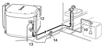
When using pressure pumps with high switching hysteresis, hot water may flow back through the cold water tap. To prevent the backflow, we recommend that a non-return valve (11 – not included in the scope of supply) be fitted between the outlet to the cold water tap and the drain valve.
