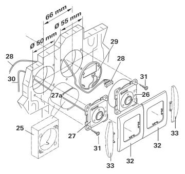
If it is not possible to install the control panels flush with the surface, Truma can provide a surface-mounting frame (25) on request, as a special accessory (part no. 40000-52600).
